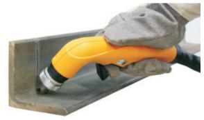
Extended consumables for cutting at inaccessible parts of workpiece
